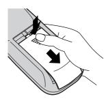
Install the batteries as shown in the battery compartment. (Polarity + or – must match the markings in the compartment.)
